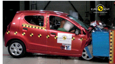
Offset crash test at 64km/h
