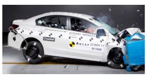
Offset crash test at 64km/h (Impreza)
