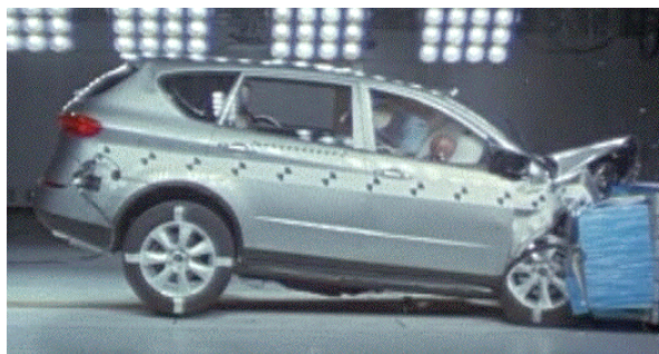
Offset crash test at 64km/h
