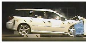
Offset crash test at 64km/h
