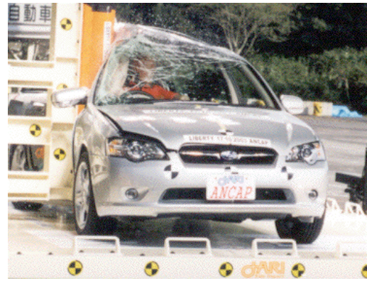
Action shot from pole impact test
