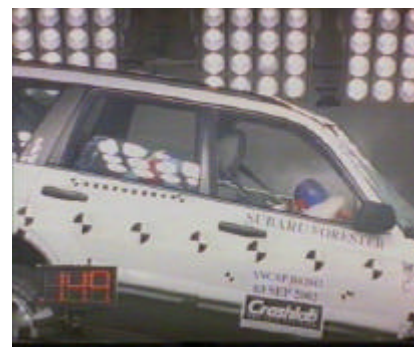
Offset crash test at 64km/h
