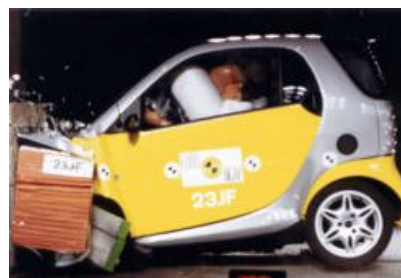
Offset crash test at 64km/h
