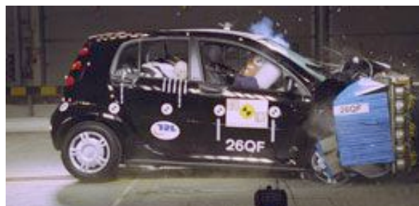
Offset crash test at 64km/h
