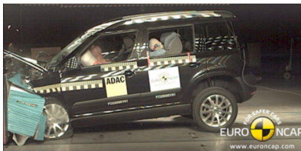
Offset crash test at 64km/h
