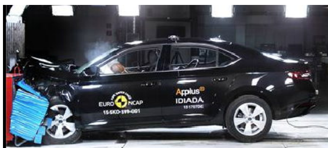
Frontal offset test at 64km/h (Copyright Euro NCAP)
