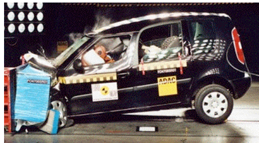
Offset crash test at 64km/h
