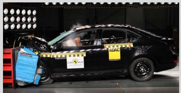
Frontal offset test at 64km/h
