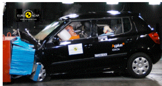
Offset crash test at 64km/h
