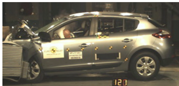
Offset crash test at 64km/h (Euro NCAP)
