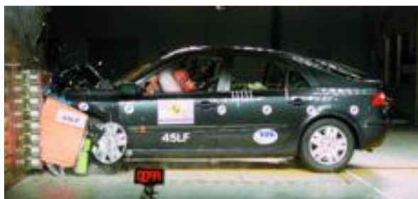
Offset crash test at 64km/h
