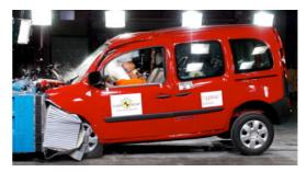
Offset crash test at 64km/h
