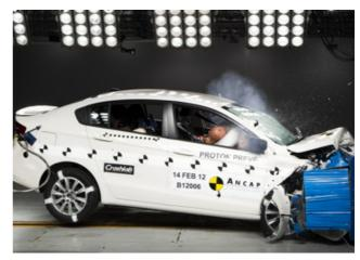
Frontal offset test at 64 km/h
