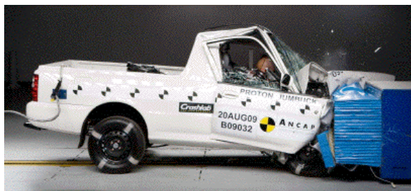
Offset crash test at 64km/h
