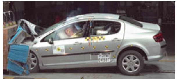
Offset crash test at 64km/h
