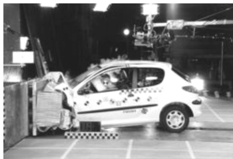
Offset crash test at 64km/h
