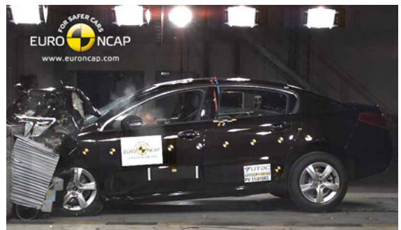
Offset crash test at 64km/h
