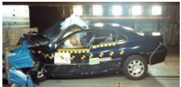
Offset crash test at 64km/h
