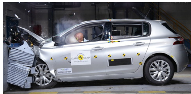
Frontal offset test at 64 km/h (Euro NCAP)
