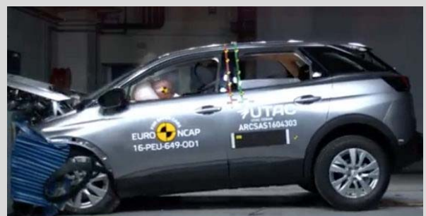
Frontal offset test at 64km/h
