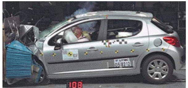
Offset crash test at 64km/h
