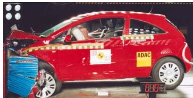
Frontal offset test at 64 km/h (Source: Euro NCAP)
