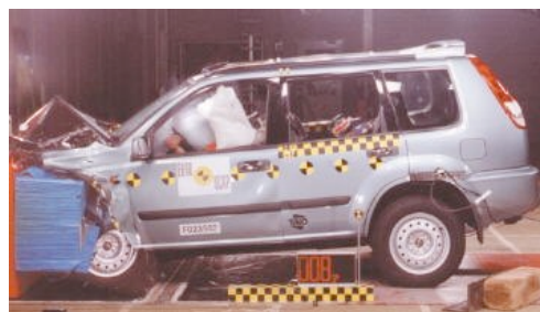
Offset crash test at 64km/h
