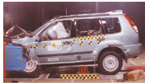
Offset crash test at 64km/h
