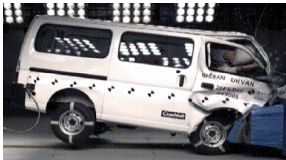
Offset crash test at 64km/h
