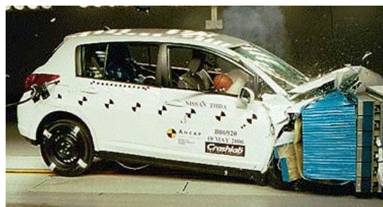
Offset crash test at 64km/h
