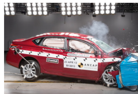
Frontal offset test at 64 km/h (sedan tested by ANCAP)
