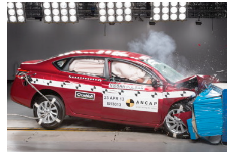
Frontal offset test at 64 km/h
