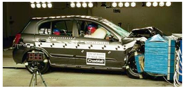
Offset crash test at 64km/h
