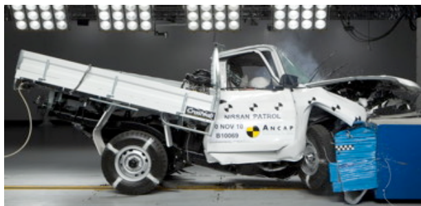
Offset crash test at 64km/h
