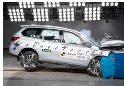
Frontal offset test at 64 km/h
