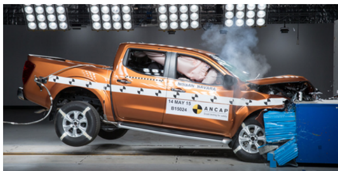
Frontal offset test at 64km/h (dual cab tested by ANCAP)
