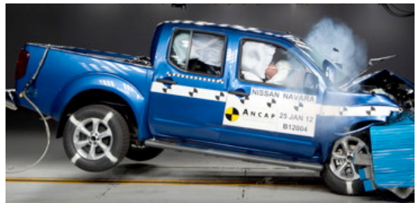
Offset crash test at 64km/h
