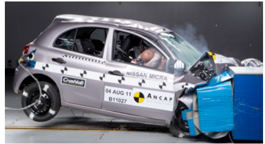
Offset crash test at 64km/h
