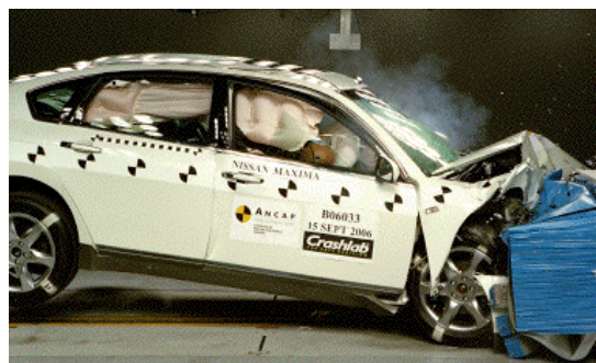
Offset crash test at 64km/h
