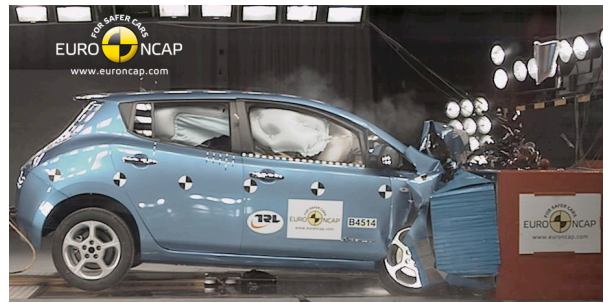
Offset crash test at 64km/h
