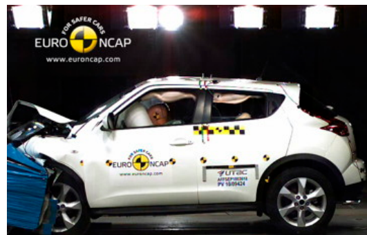
Frontal offset test at 64 km/h (Euro NCAP)
