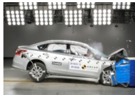
Frontal offset test at 64 km/h
