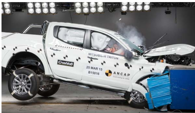
Frontal offset test at 64km/h
