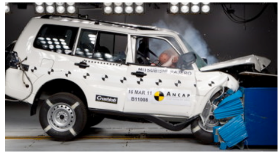
Offset crash test at 64km/h
