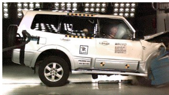
Offset crash test at 64km/h
