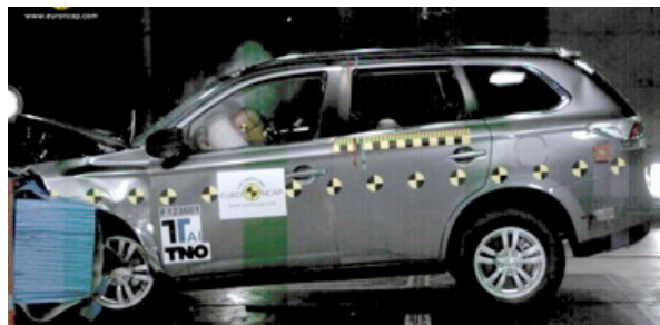
Offset crash test at 64km/h (Euro NCAP)
