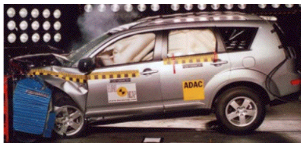
Offset crash test at 64km/h
