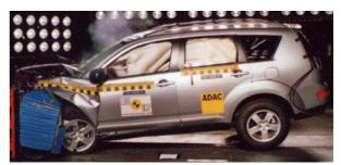
Offset crash test at 64km/h
