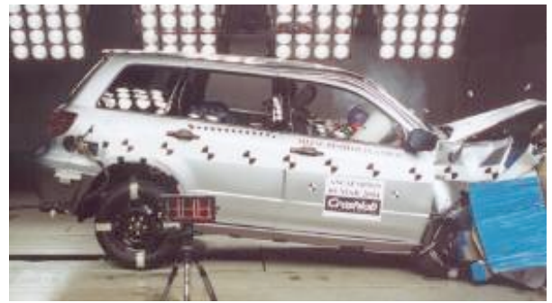
Offset crash test at 64km/h
