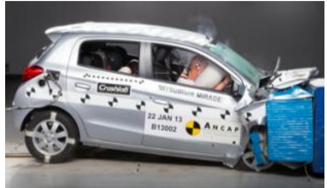
Frontal offset test at 64 km/h
